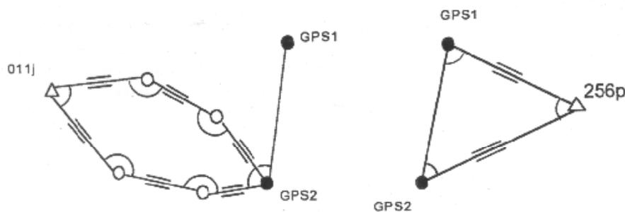
Fig. 2. Examples of tying of GPS points to points of classical horizontal network using classical measurements
