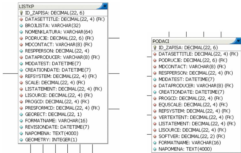
Figure 4. Design of tables used for storing metadata about map sheets and all the other data sets
