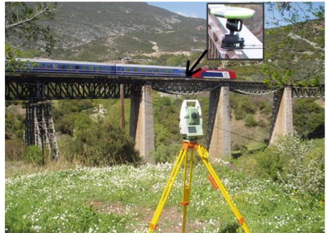
Figure 1. The Gorgopotamos Railway Bridge and in the foreground the RTS used for the measurements focusing on reflector at a midspan. An inset shows the prismatic reflector and on top of it the antenna of a GPS, used as a chronograph.
