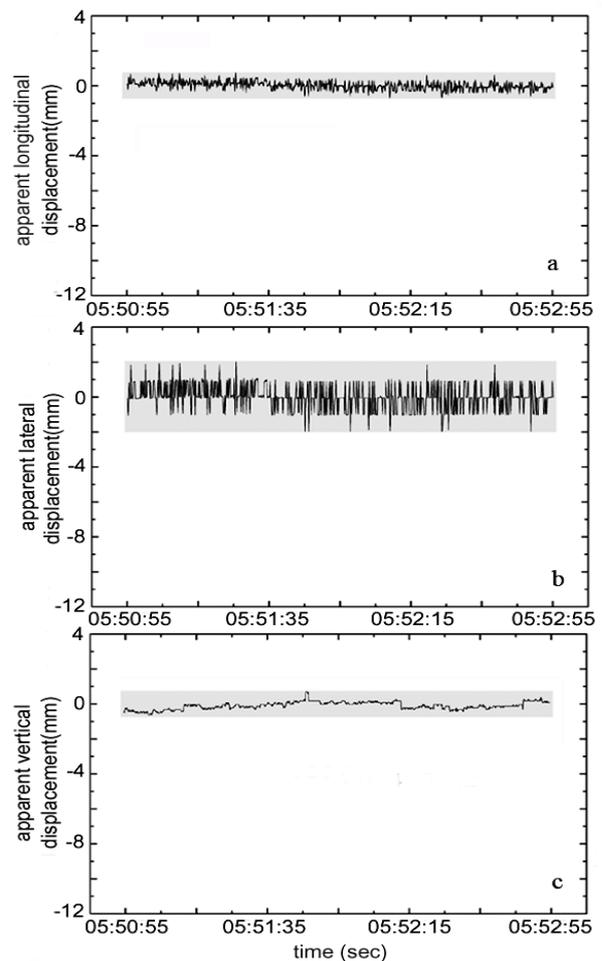
Figure 2: Time series of apparent displacements along the longitudinal, lateral and vertical axes corresponding to the point over the pylon, while no train was passing. The noise level (shaded zone) in the vertical axis was  $\pm 1$ mm, but along the lateral axis  $\pm 2$ mm, probably because of wind-induced lateral oscillations of the handrail of the bridge.
