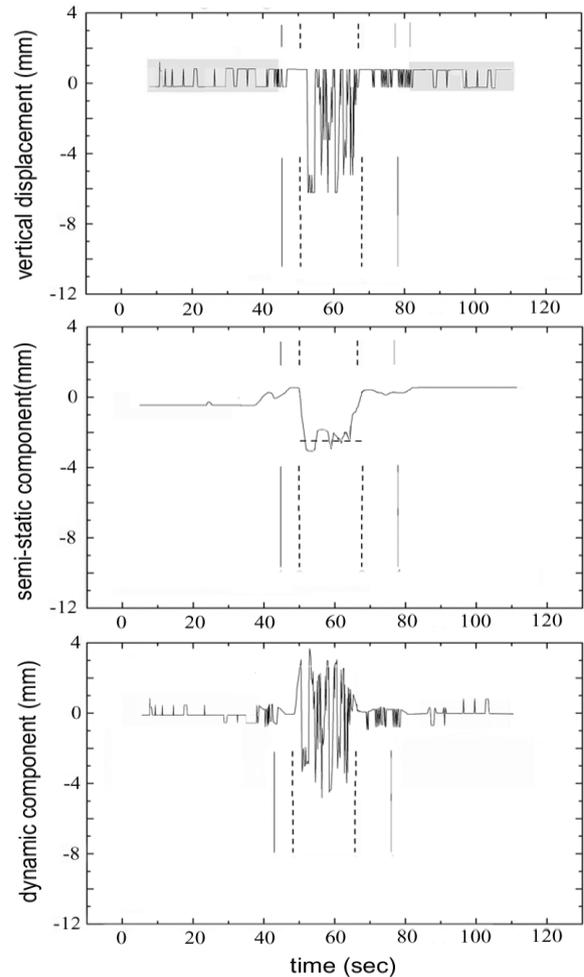
Figure 4. Decomposition of the apparent vertical displacements (top) into long (middle) and short-period components (bottom), corresponding to semi-static and dynamic displacements. Shading indicates noise.
