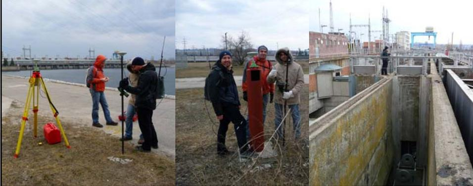
The site survey is an important operation consisting of validating the existing geodesy (coordinate system), the designed location of instrumentation (GNSS and TPS) and to obtain information for the final design validation using "Least Squares Simulation" processing.
