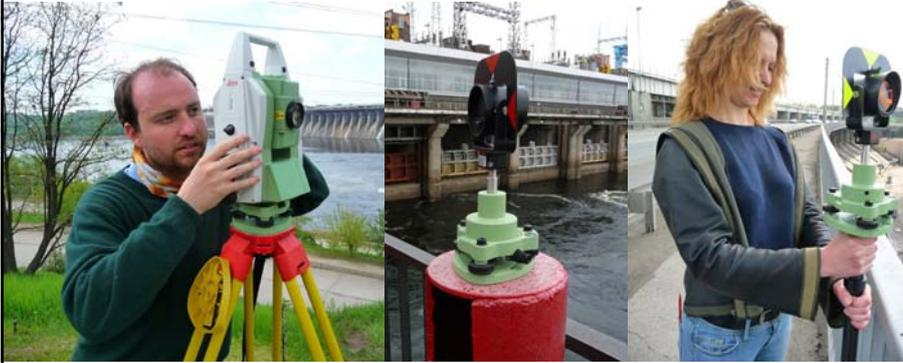
The site survey with TPS is an important operation consisting of validating the designed location of instrumentation (TPS and Reflectors), the performances on site and to obtain information for the final design validation using "Least Squares Simulation" processing.
