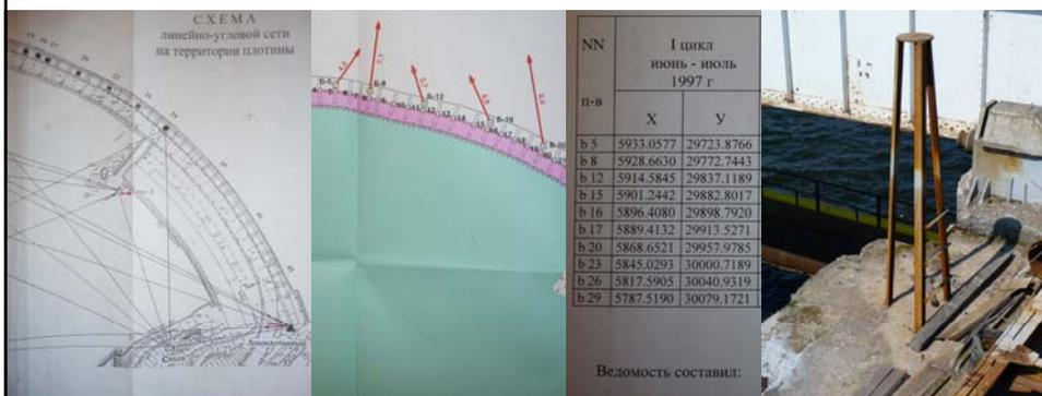
Previous Geodetic Monitoring Campaign executed by University, Geodesy Department using GPS on pillars. Control points and monitoring points on steel pillars anchored on massive concrete foundations.
