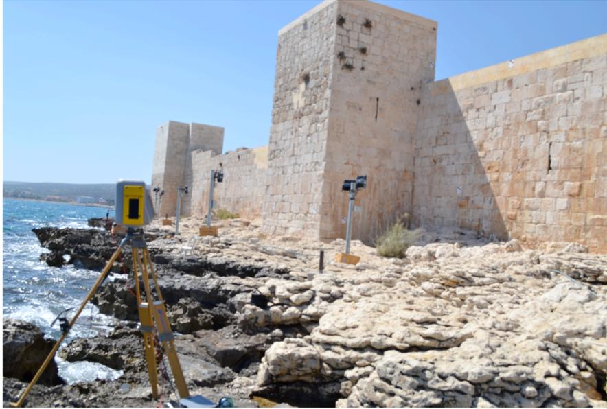
**Image 10: Topographic Laser Scanning Operation (Ulvi A. ,2012)**
