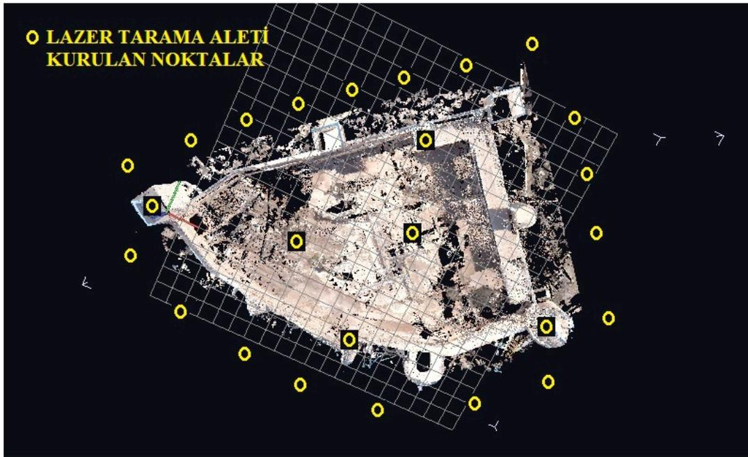
**Image 12: Scanned Stations of laser scanning Trimble GX 3D**
