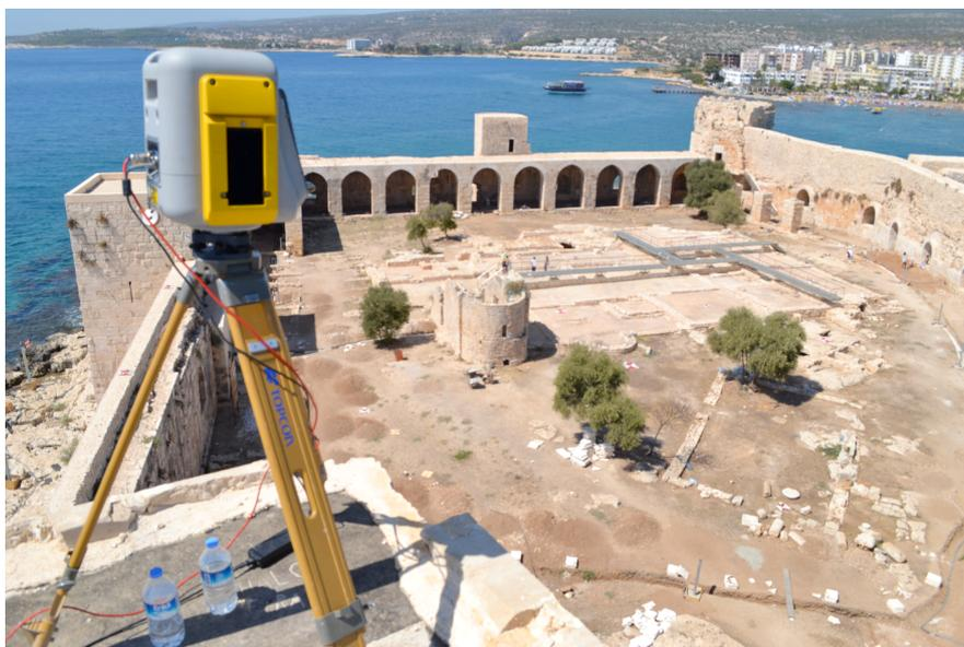
**Image 9: Topographic Laser Scanning Operation (Ulvi A. ,2012)**
