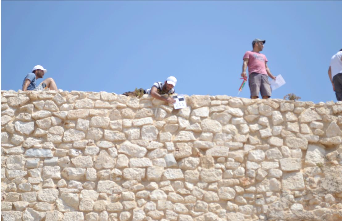
**Image 7: Attachment of paper targets to wall (Ulvi A. ,2012)**
